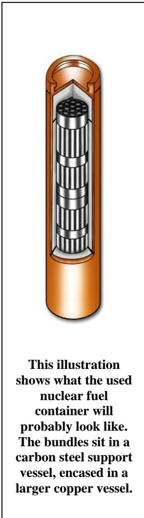
**This illustration shows what the used nuclear fuel container will probably look like. The bundles sit in a carbon steel support vessel, encased in a larger copper vessel.**
