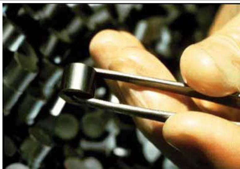
**Uranium dioxide is pressed and heated to extreme temperatures to produce ceramic fuel pellets, like the one shown here. These pellets are extremely durable and strong.**
