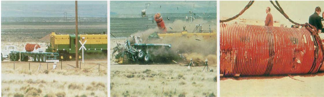
**Figure 1:** These images illustrate the kind of tests done on used nuclear fuel shipping containers. The transport truck stops on the railroad tracks to simulate a stalling scenario, while a fast moving train slams into the flatbed directly. The shipping container is slightly damaged, but the contents remain contained.
