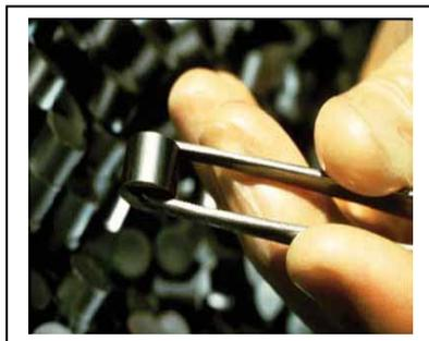
**STEP FOUR – FABRICATION:** The uranium dioxide is sent to one of two fabrication facilities, either in Port Hope or Peterborough, Ontario, where it is pressed and heated to extreme temperatures to form ceramic pellets. The pellets are placed into long tubes which are bundled together into an assembly called a fuel bundle. The fuel bundle is about the size and shape of a
