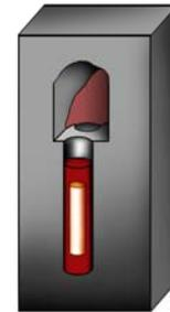
This image shows how the container may be placed into the host rock of the DGR.
