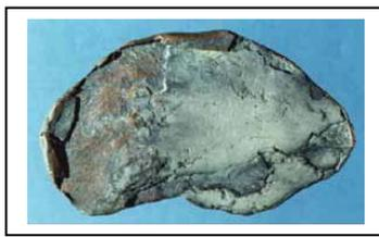
Under deep rock conditions copper is extremely durable and resistant to various types of corrosion. Copper is one of the few metals found in its native state in the geological environment, and studies on natural
